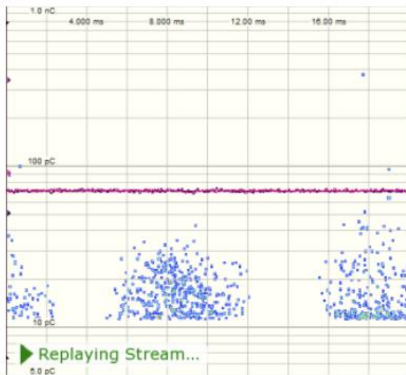
OHL terminations – HFCT sensor @2MHz
